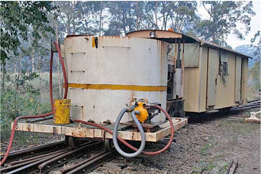
The new fire train undergoing on track testing : ex-Moreton Mill water and mill bridge gang (used as a crew room) wagons during the fire training day. Note the new pump and hose attachment. Paul Rollason photo [img4934-2]
