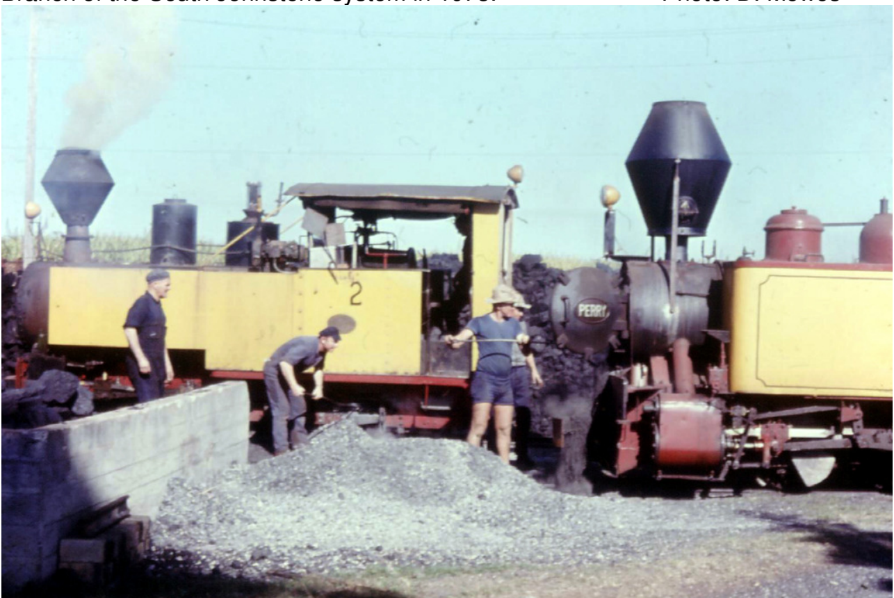
Delta has her ash removed from her smokebox while Invicta simmers by quietly, 1970. Photo: D. Mewes
