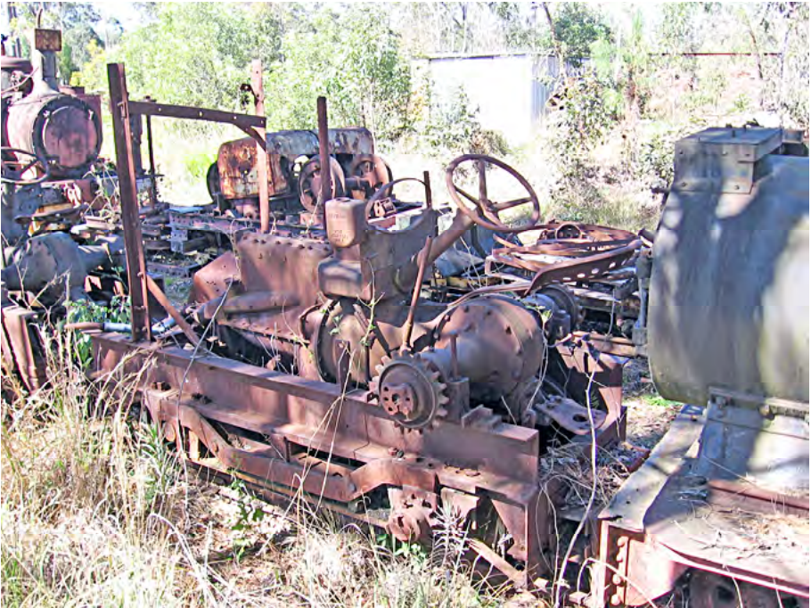
The second Caledonian Colliery Fordson Rail Tractor at Woodford; remains of the framework that held up the metal canopy can be seen. Greg Stephenson photographer.
