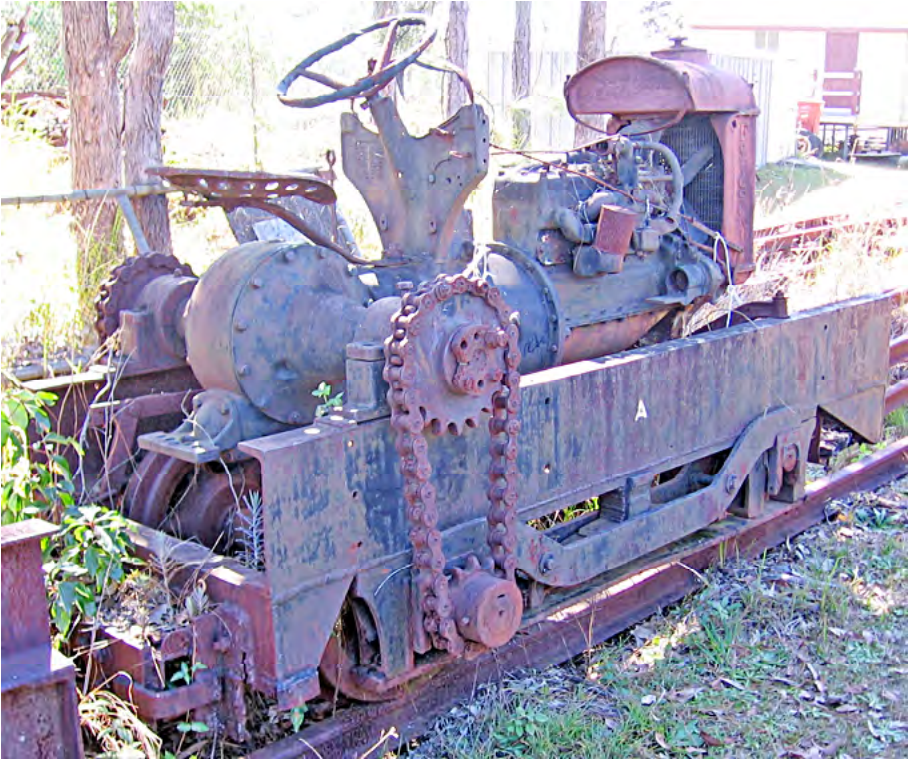
1938 Fordson Rail Tractor with chain drive between the rear axles. Another chain drive down the centre of the rail axles connected the four wheels. Greg Stephenson photographer.
