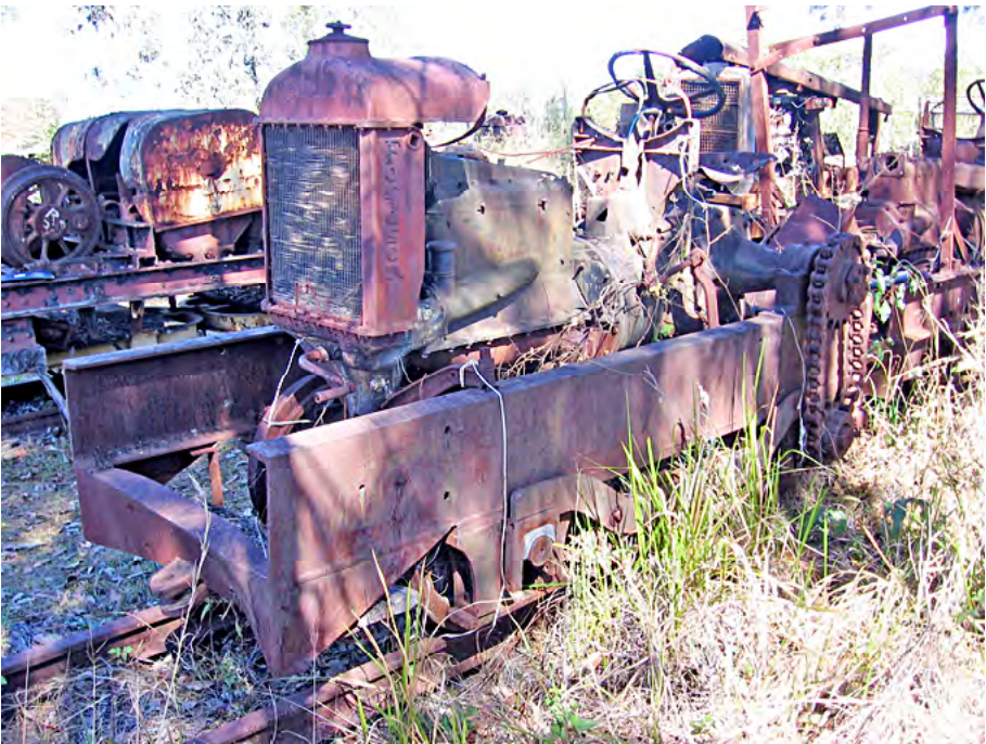
One of the two Caledonian Colliery Fordson 4wPM (chain drive) Rail Tractors at Woodford. Both were built by Forrers Pty Ltd of Ipswich using Fordson 4 cylinder tractors. Details inside. Greg Stephenson photographer.
