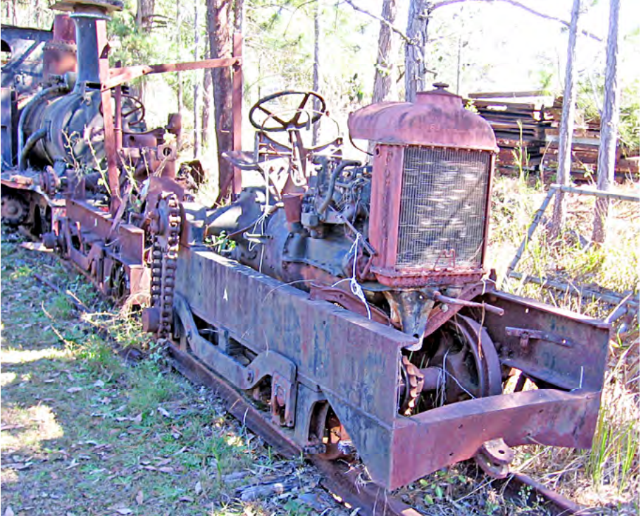
The two Fordson Rail Tractors (Forrers Pty Ltd, Ipswich, 22 hp, 1928 and 1938) that operated at Caledonian Colliery at Thagoona before coming to ANGRMS. Greg Stephenson, photographer 2008.
