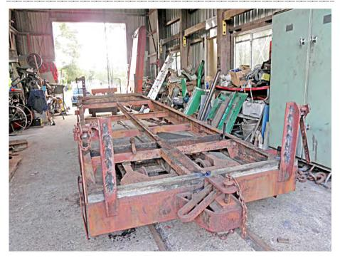
Ex-Moreton Mill bogie open wagon during refurbishment for use as an extra maintenance wagon. Rotten timber has been removed and replacement timber ordered. Bob Gough photographer.
