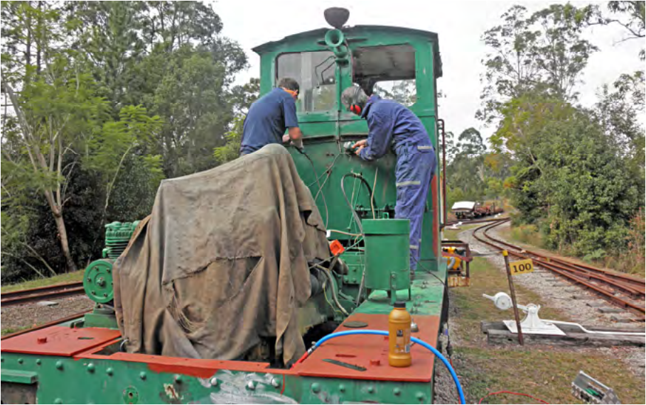
Wayne Harman and Ray Sergent removing green paint and rust from the Baguley. Bob Gough photographer.
