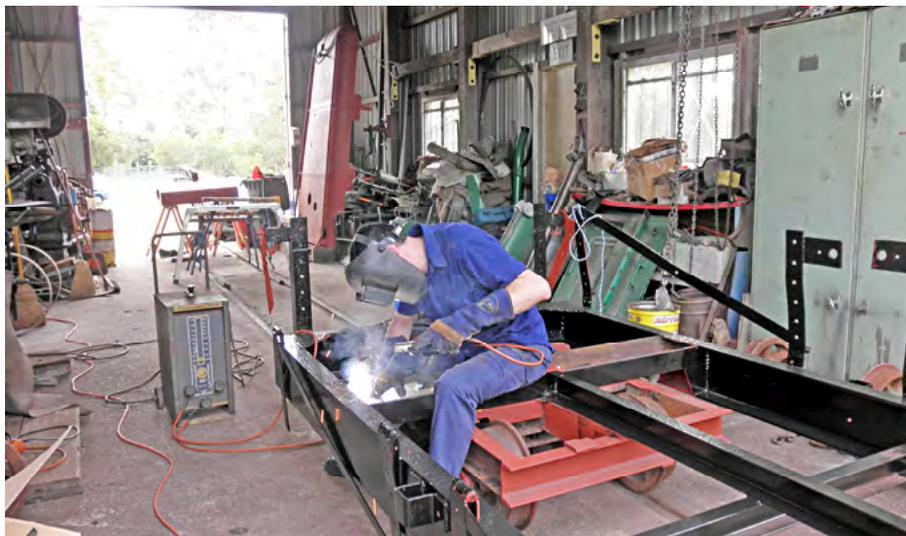
Mark Gough replacing rusted sections on the Nambour work wagon. Bob Gough photographer.
