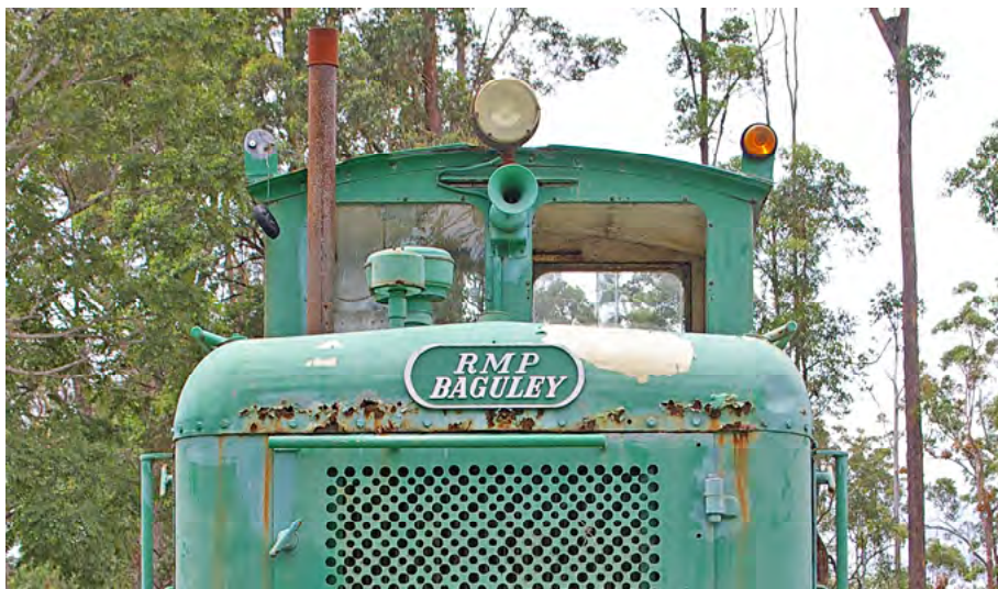
RMP Baguley showing the extent of rust on the bonnet. Brian Webber photographer.
