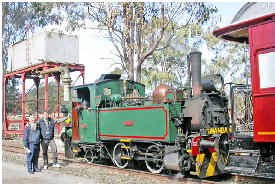
Kilrie, ex-Pioneer Sugar Mill, (3' 6" gauge, 0-4-2T, Perry #265, 1924) overshadowed by the QR heritage carriages it is hauling at the Queensland Pioneer Steam Railway, Swanbank, 6 Aug 2006. Kilrie was once part of the ANGRMS' fleet and is now owned by QPSR. Lynn Zelmer photographer
