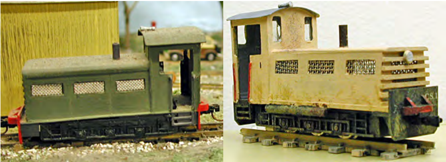
Bob Dow's Jenbach model (left), Lynn Zelmer's (right). Both are HO N 30, built from styrene, and use Bachmann N scale mechanisms.
