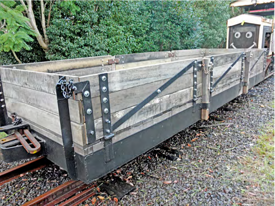
The Moreton Mill bogie open wagon, now restored and ready for accreditation. Bob Gough photographer.
