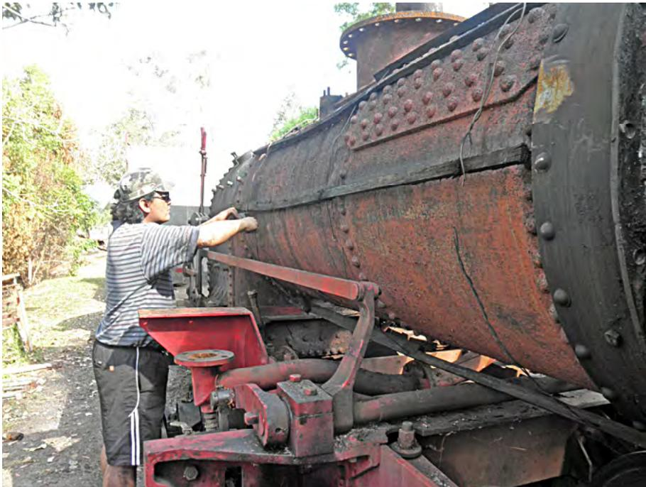
Brad Bell removing cladding support timbers from Bundy's boiler during the work party, 29 September 2012. Bob Gough photographer.
