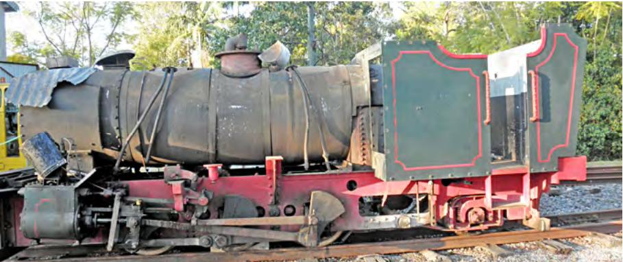
Bundy with the boiler cladding and cab removed late September. At this point the boiler was ready to be lifted from the frame for retubing; with a new smoke box, new internal steam pipe, boiler thickness test, new brake blocks and other work to be done as needed. Bob Gough photographer.
