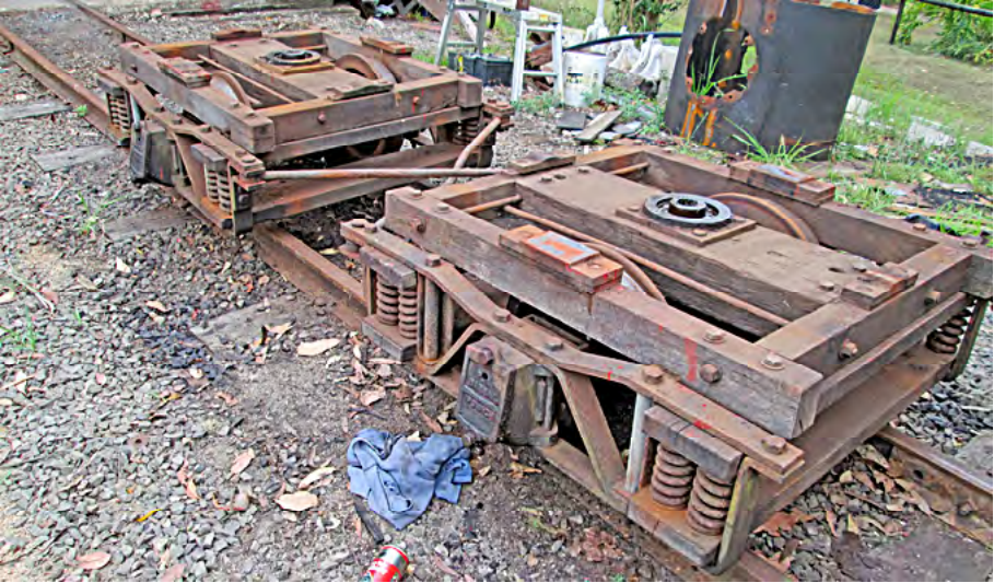
Grover's bogies, connected together but without the wagon frame, showing the crossed arms which cause the bogies to steer around corners, December 2012, Ryan Silk photographer. [rs_0217]
