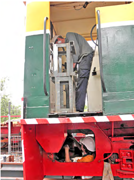
Above left: Mark Gough in cab and Ryan Silk in the pit removing Netherdale's brake cylinders. Bob Gough photographer. Above right: Alex Perkins standing in the pit and holding onto the winch rope that made life so much easier for the removal of the brake cylinders. Mark Gough photographer.
