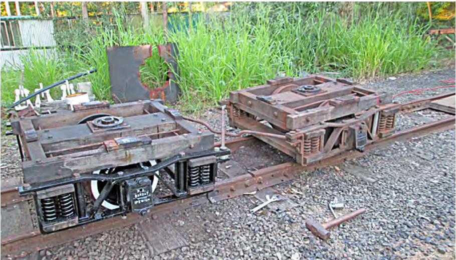
One of the Grover's wagon bogies rebuilt, mid-April. Ryan Silk photographer.
