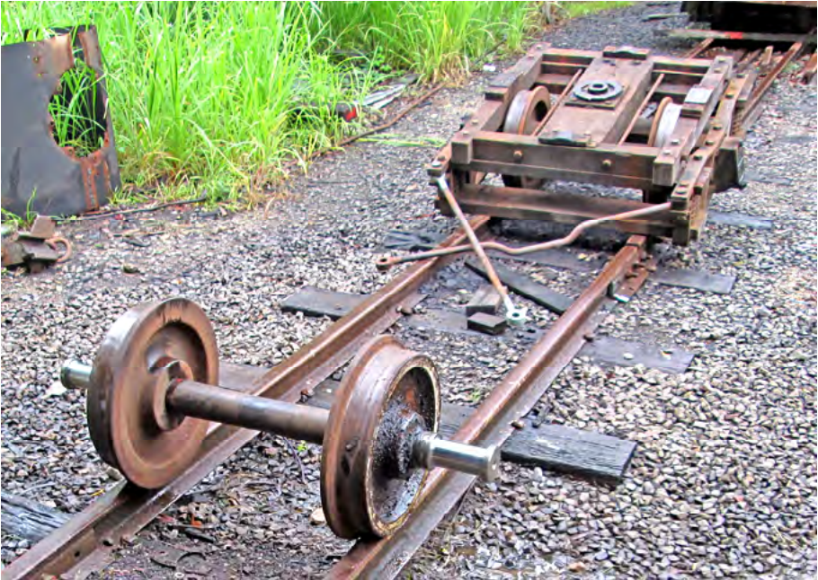
Grovers bogie wagon wheel set, disassembled with work being conducted on the entire bogie frame. Ryan Silk photographer.
