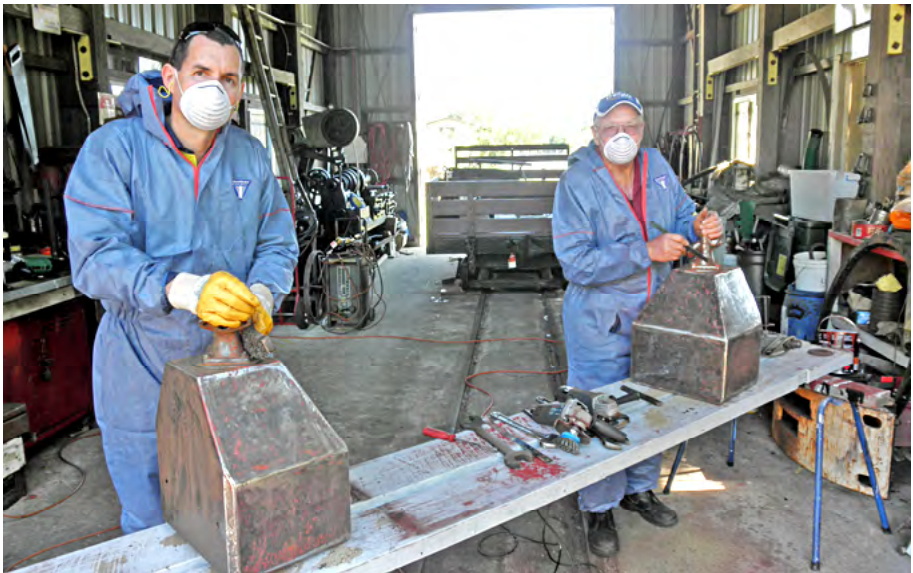
Mark and Bob Gough removing paint and rust from Netherdale's sand boxes prior to undercoating, 7 Sep 2013. Ryan Thomas photographer
