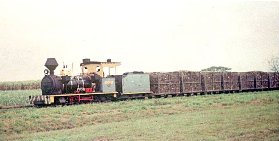
A sister locomotive to ANGRMS' Melbourne, Sydney (0-6-0 Hudswell Clarke of Leeds #1838, 1950) heading to the mill with a rake of full cane bins, likely during the first year Victoria Mill operated only with cane bins, c1970. Bill Blannin photographer.
