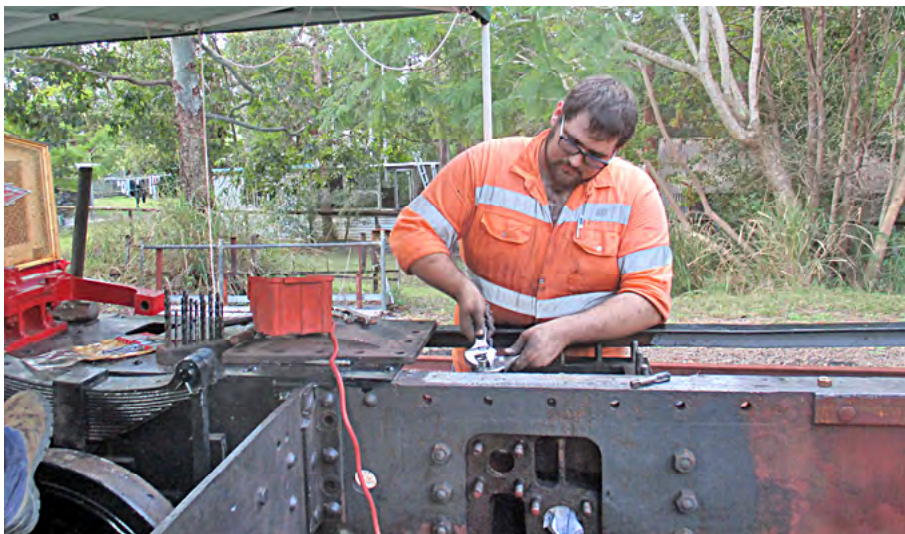
Tyler fitting new studs to the fireman's side. Ryan Silk photographer.
