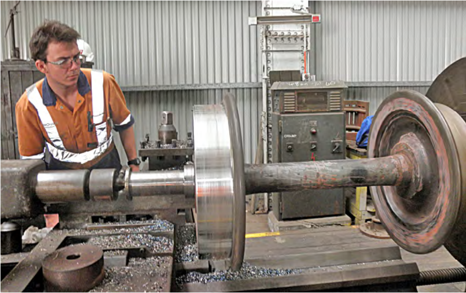
Ryan Silk machining the Pony truck wheels, May 2015. Bob Gough photographer.
