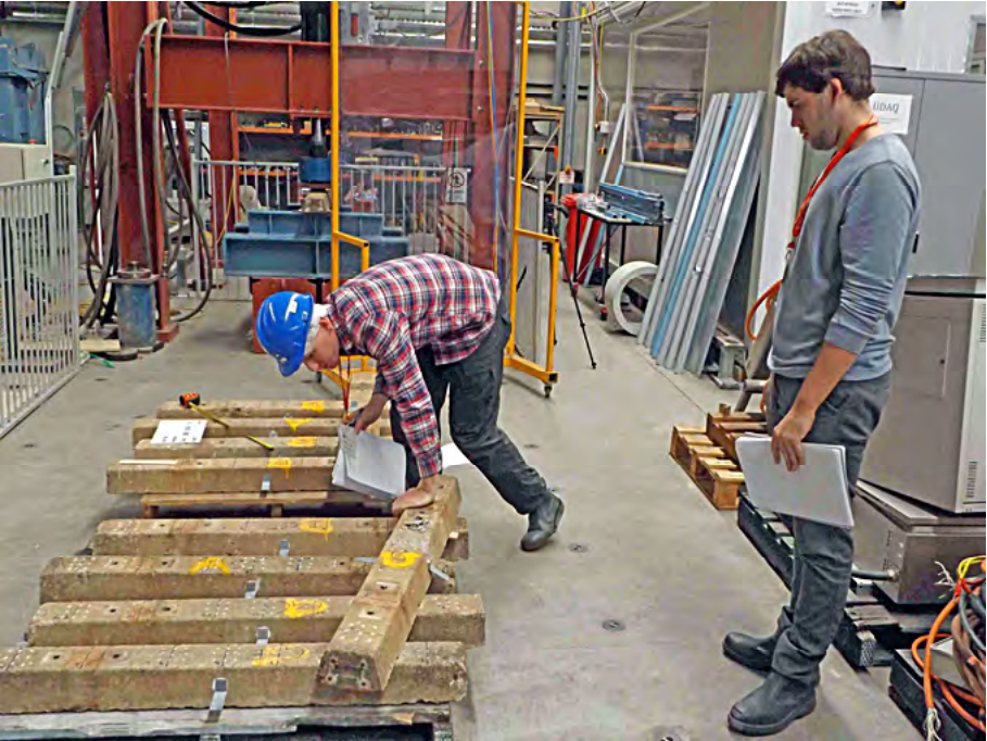
QUT students Daniel Dwyer inspects tested concrete sleepers to understand the mode of failure and performance whilst Nathan Davey looks on. Greg Stephenson photographer.
