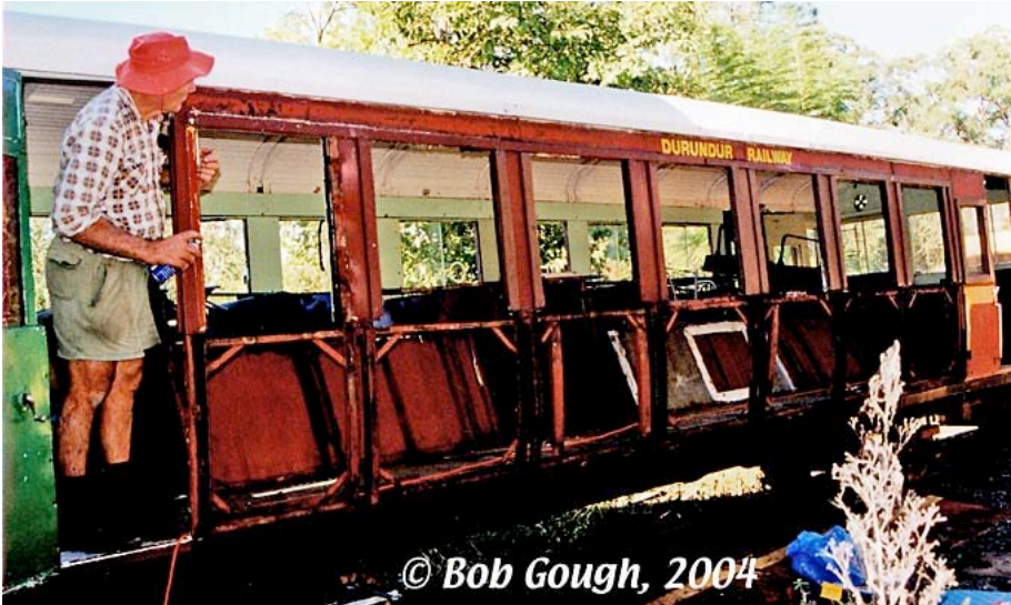
Side removed from PL111 for necessary repairs, details in Greg Stephenson's Track Matters. Bob Gough photo.
