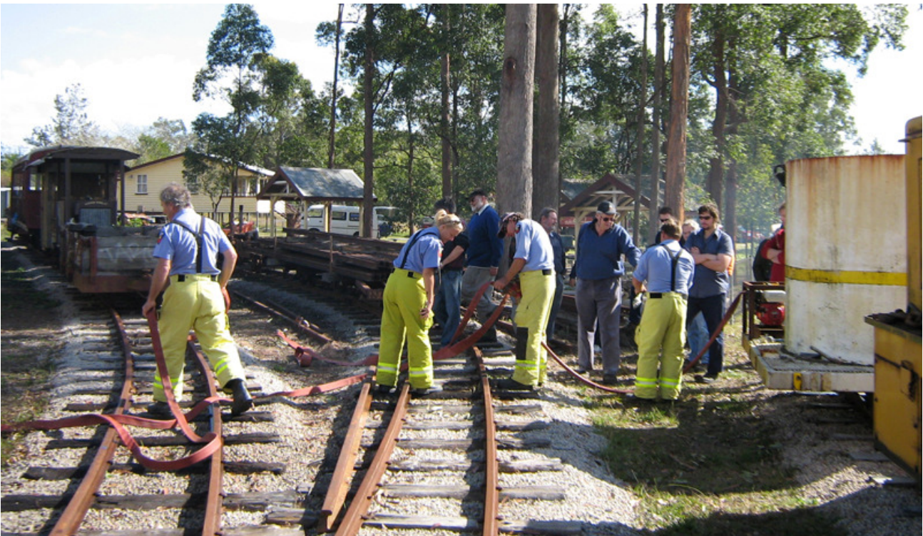
The Woodford Fire Brigade members couple their hoses and branches to our pump and tank wagon to check the compatibility equipment - Photo: B.Blannin
