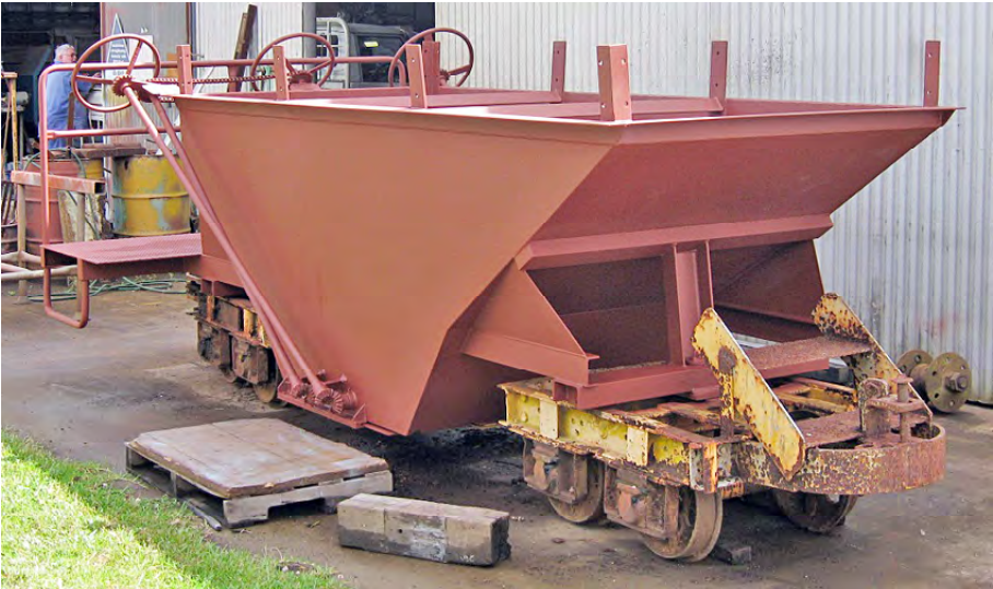
Progress to date (November 2010) on rebuilding the ballast wagon at Hewitts Engineering. Terry Olsson photo.
