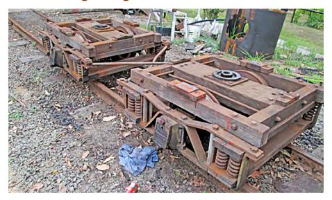
Grover's bogies, connected together but without the wagon frame, showing the crossed arms which cause the bogies to steer around corners, December 2012, Ryan Silk photographer. [rs 0217]
