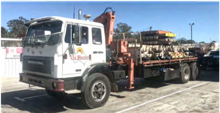
Greg Adams crane truck at Apple Tree Creek with new concrete sleepers for ANGRMS, 15 April 2021. Terry Olsson photographer.
