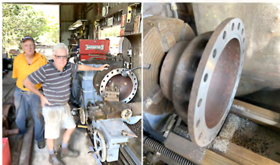
Bob Gough (left) and Mick Ewer after the machining of the sealing surface of the Perry's steam dome, the lathe in the workshop making this an easy job. May 2021, Mark Gough photographer.
