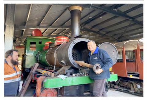
Laurie Erb removing the Perry's internal steam pipe, Ryan looking on. The male end of the pipe has deteriorated over time and was unable to make good seal with the female part of the new regulator when tested, so a new piece will be made and fitted. 11 July 2021. Mark Gough photographer.
