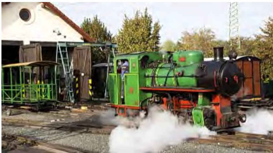
"Kacka" 0-4-0T Steam Locomotive BS 80 in the loco shed. Built in 1951 by CKD Sokolovo Praha Liben. KSBR website.
